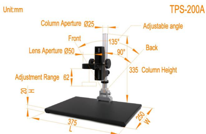
Figure 9-14 TPS-200A. TPS-200B can be obtained by rotating base B20A 90 degrees(B20B) and assembling it with bracket A20
