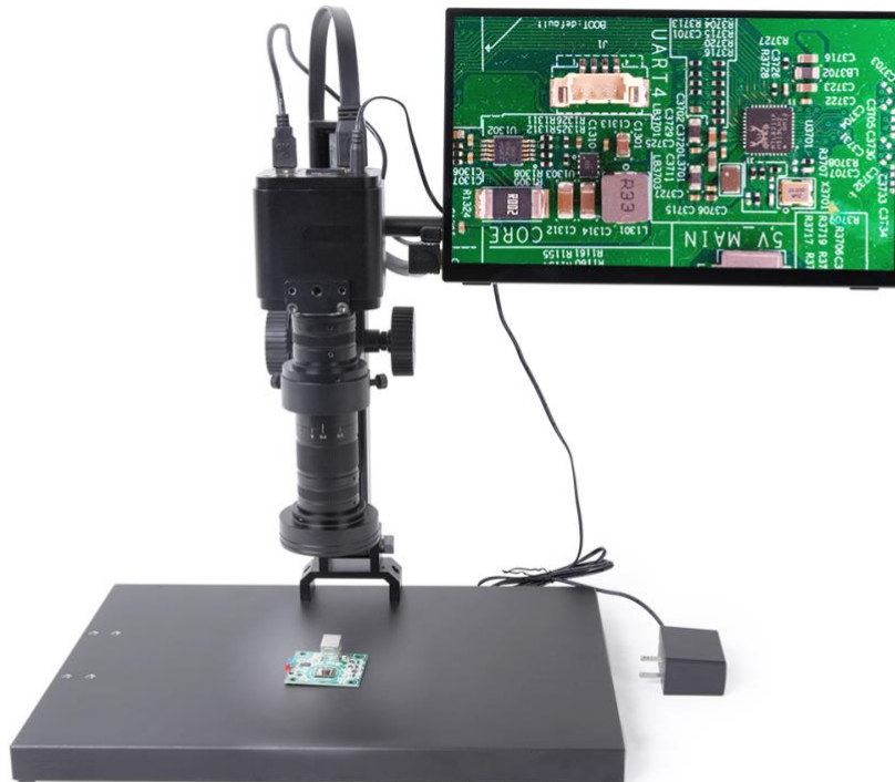
Figure 8 TPS-210A50-G(Stand)+TzM0480 (0.4x-8.0x Monocular Zoom Objective) +TXCAMLITE4K Camera(HDMI/USB Output CMOS Camera with Touch Function)+Touch Screen, the Touch Screen Is Fixed on the Cross Bar of Stand through the Mounting Hole on the Built-in Bracket (Front View, Short HDMI Cable and USB Type A to Type C Data Cable Can Be Used to Connect the Camera and Touch Screen)
