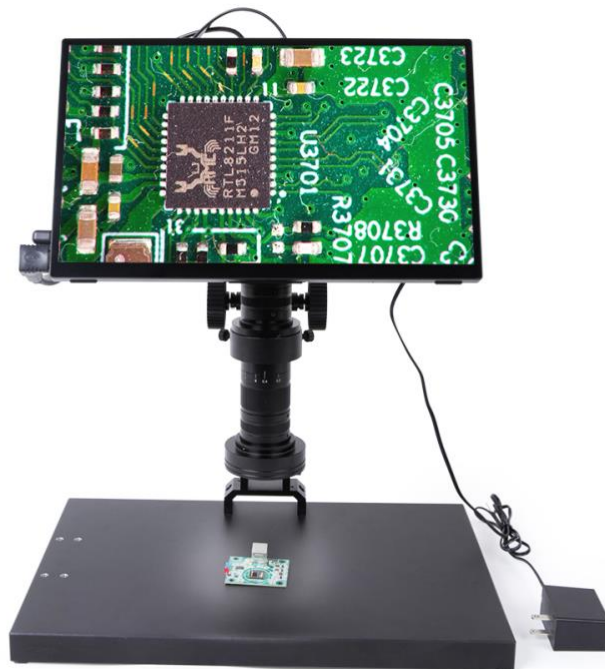
Figure 6 TPS-210A50(Stand)+TZM0480 (0.4x-8.0x Monocular Zoom Objective) +TXCAMLITE4K Camera(HDMI/USB Output CMOS Camera with Touch Function)+Touch Screen, the Touch Screen Is Fixed on the Fixing Block at the Front of the Camera through the Mounting Hole on the Built-in Bracket (Front View, Short HDMI Cable and USB Type A to Type C Data Cable Can Be Used to Connect the Camera and Touch Screen)
