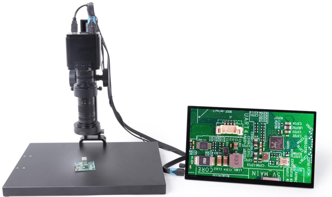
Figure 5 TPS-210A50(Stand) + TZM0480(0.4X~8X Monocular Zoom Objective) + TXCAMLITE4K(HDMI/USB Output CMOS Camera with Touch Function) + Touch Screen, the Touch Screen Can Be Tilted on the Table Through Its Own Stand (Long HDMI Cable and USB Type A To Type C Data Cable Are Required To Connect the Camera and Touch Screen)
