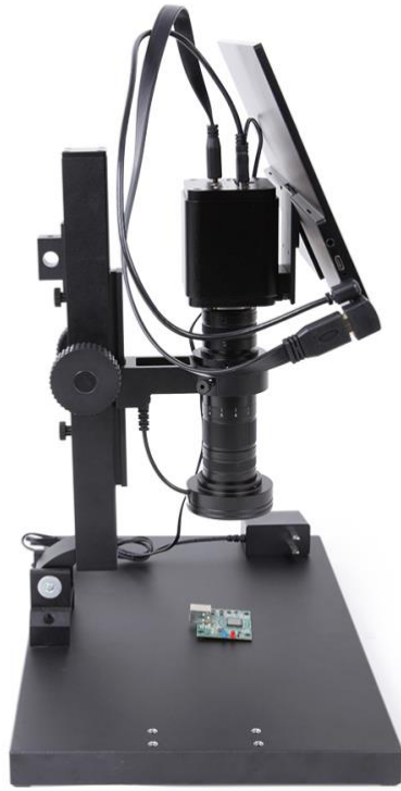
Figure 7 TPS-210A50(Stand)+TzM0480 (0.4x-8.0x Monocular Zoom Objective) +TXCAMLITE4K Camera(HDMI/USB Output CMOS Camera with Touch Function)+Touch Screen, the Touch Screen Is Fixed on the Fixing Block at the Front of the Camera through the Mounting Hole on the Built-in Bracket (Left side View, Short HDMI Cable and USB Type A to Type C Data Cable Can Be Used to Connect the Camera and Touch Screen)
