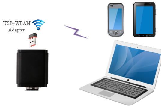
Figure 6 The PC or Mobile Device Connect to the Camera through WLAN
