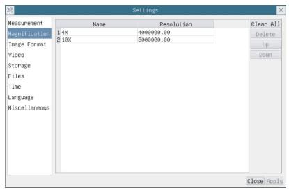
Figure 8 Comprehensive Magnification Calibration Settings Page
