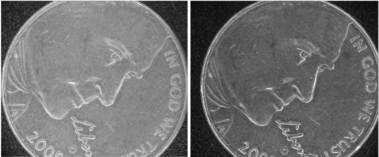
Figure 8-46 Ordinary camera (left) compared with polarizing camera (right) metal surface effect
