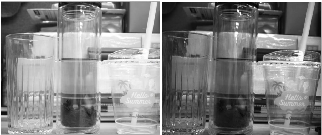
Figure 8-44 Comparison of plastic surface effects between ordinary camera (left) and polarizing camera (right)
